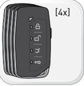
[4x] **WARNING:** Complete the module programming procedure and tach programming procedure before programming the remotes. A maximum of four [4x] remotes per system.
