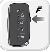
To program an additional remote as second vehicle mode: Follow steps 1 to 4. Press twice [2x] on the "F" button then press once [1x] on the LOCK button of the remote. Follow steps 6 to 9.
