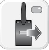
Release the antenna button. The antenna's leds will turn OFF.
